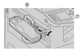
5 Place the handset (③) on the handset cradle, then connect the handset cord (⑥) to the handset.
